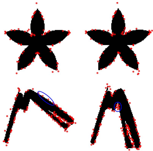
Fig. 7. Stability of support vectors with respect to variation of RBF kernel width (\gamma) and articulation. Top: Support vectors when \gamma varies. \gamma = 0.0027 in the first shape and \gamma = 0.0054 in the second shape. Sixty-two out of 78 support vectors in the first shape appear in the second shape. The overall positioning of the support vectors is very similar. Bottom: Support vectors with shape articulation. Blue circles indicate SVs that do not have correspondences on the other shape. Eighty-three out of 114 SVs in the first shape appear in the second shape.
